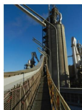
A 30 t/h HOTDISC installed at Arabian Cement for the combustion of alternative fuels can achieve a thermal substitution rate of up to 40%.
