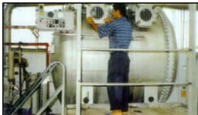
Checking peroxide concentration with tester after enzyme bleach clean up
