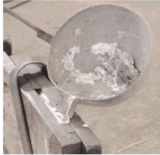
Pouring molten aluminium into slabs for rolling
