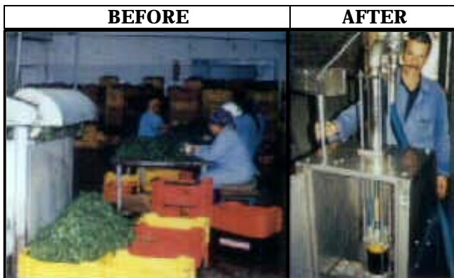
Semi-automatic vegetable paste packing has eliminated handling losses
