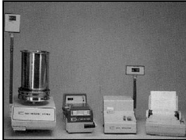
Figure 6.1: Illustration of an Automatic (Electronic) Milk Collection System 75
