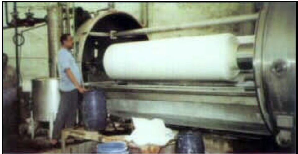
Production scale trials for desize and scour at Misr Beida Dyers
