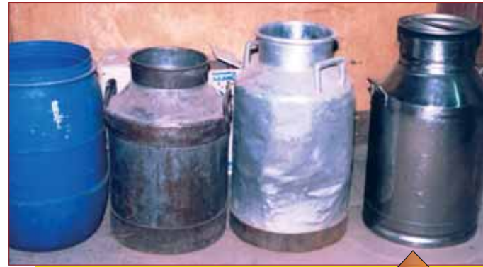
Recommended stainless steel milk collection can
