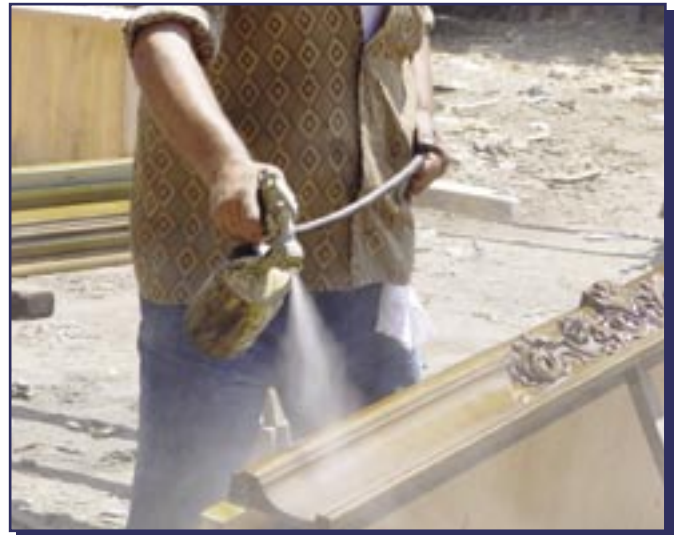
Furniture spraying using conventional spray gun
